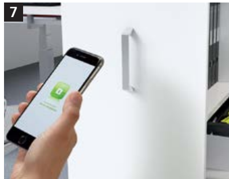
7 RFID lock with Bluetooth Reading range up to 10 m
