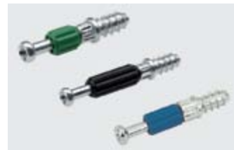
Coloured plastic sleeves in easy-grip fluted design indicate dowel length. Green (dowel length 20 mm) for Rastex 15, blue (dowel length 24.5 mm) for Rastex 25 and black (dowel length 30 mm) for Rastex 15.
