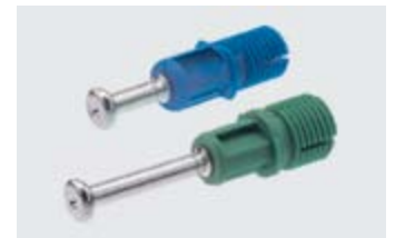
Fits into the hole in the carcase side quickly and easily without the need for tools. Easy to tell apart with coloured expanding elements for 8 mm (blue) and 10 mm (green) drill holes.
